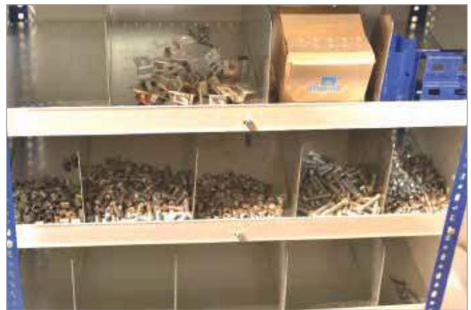
Store. Stop spilling over...!! : Front stopper strips hold back the contents of the storage partitions from spilling over.
