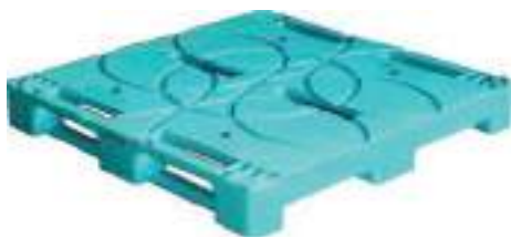
Model : AP1111SC Dimensions : 1100 (L) x 1100 (W) x 140 (H) mm. sprox. Load Bearing : Uniformly Distributed Load Static : 3600 kg. • Dynamic : 1200 kg. • Racking : 600 kg. Should be handled with Forklift or Pallet truck only.
