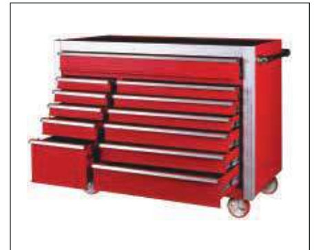
Model : NKTB8312-DX Overall Dimensions : 1412 x 745 x 947 mm. Package : 1474 x 838 x 1280 mm. Dimensions With Castors : 1412 x 745 x 1176 mm. 1 drawer : 1229.5 x 675 x 123 mm. 3 drawers : 371 x 675 x 79 mm. 1 drawer : 371 x 675 x 107 mm. 1 drawer : 371 x 675 x 275 mm. 3 drawers : 777 x 675 x 79 mm. 2 drawers : 777 x 675 x 107 mm. 1 drawer : 777 x 675 x 163 mm.
