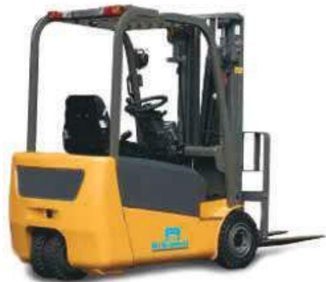
Model : NK15E3W Capacity (kg) : 1500 • Lift Height up to (mm.) : 6000
