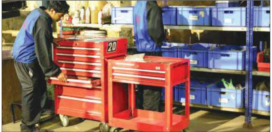
Model : NKTC333-X Overall Dimensions : 712 x 440 x 694 mm. Dimensions With Castors : 712 x 440 x 814 mm. Package : 746 x 462 x 348 mm. 2 drawers : 570 x 395 x 60 mm.
