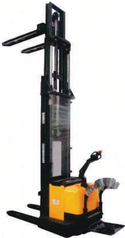
Model : NKES1232 / 1529 / 1536 / 1546 / 1560 / 1563 Capacity (kg) : 1200 & 1500 • Lift Height (mm) : 2900 to 6300
