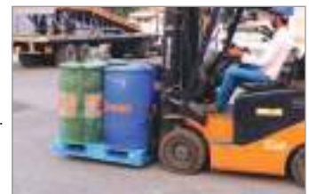
Model : DP1212 Dimensions : 1200 (L) x 1200 (W) x 150 (H) mm. sprox. Load Bearing : Uniformly Distributed Load Static : 6000 kg. • Dynamic : 1500 kg. • Racking : 1000 - 1500 kg. Should be handled with Forklift only.
