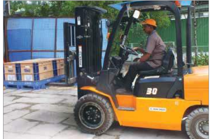
Model : NK20D / NK30D • Capacity (kg) : 2000 / 3000 • Lift Height upto (mm.) : 6000 • Mast : 2 Stage / 2 Stage FFL / 3 Stage FFL
