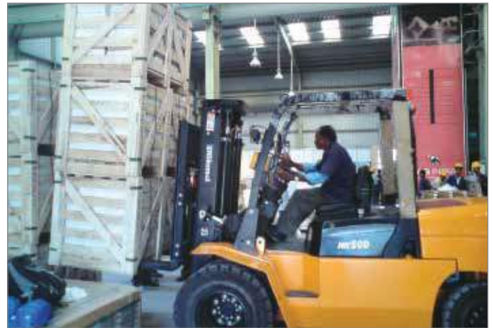
Model : NK50D • Capacity (kg) : 5000 • Lift Height upto (mm.) : 6000 • Mast : 2 Stage / 2 Stage FFL / 3 Stage FFL
