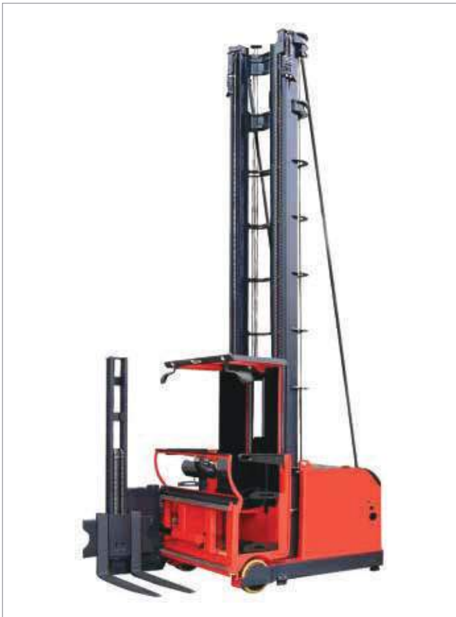
MAN-UP TURRET TRUCKS (Very Narrow Aisle - V.N.A.) (7 Models available) • Lift height up to : 9000 mm.-170000 mm. • Lift Capacities up to : 1100-2000 kg.
