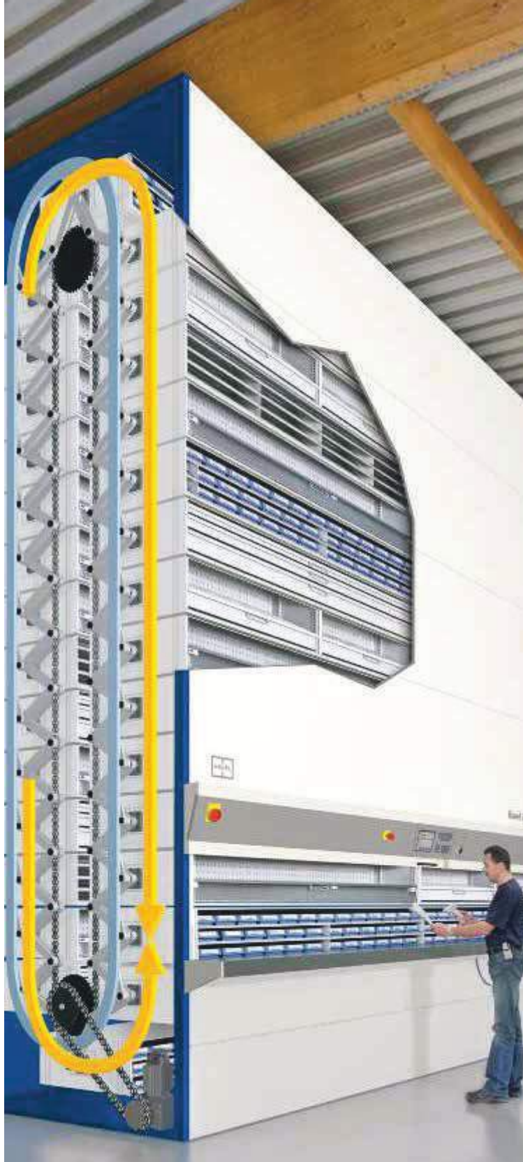
RotoMat Operating Principle
