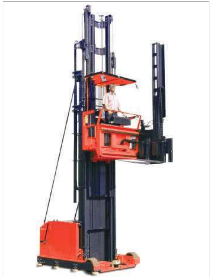
MAN-UP TURRET TRUCKS (Very Narrow Aisle - V.N.A.) (7 Models available) • Lift height up to : 9000 mm.-170000 mm. • Lift Capacities up to : 1100-2000 kg.
