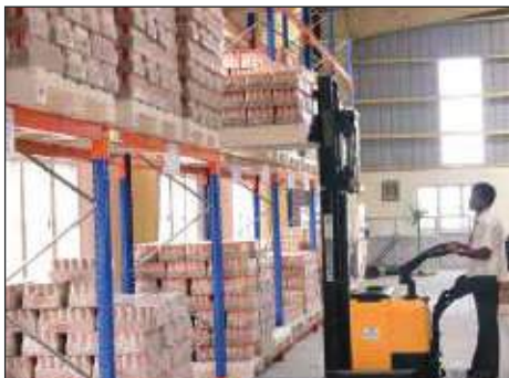
Electric Stacker moving pallet from the rack
