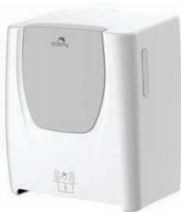
DPDR0068 Automatic HRT Tissue Paper Towel Dispenser Material : ABS Plastic Operations : Infrared Sensor, Adjustable dispense length Power : Electricity + Battery (4 X D Size Duracell Battery-Not Included) Size : 290 x 220 x 363mm Paper Roll Size : Width 195-200mm Dia : Ø 200mm/37GSM
